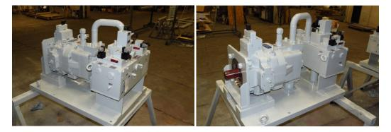
**For sizes D150 and over**, Oilgear <u>replacement Kits with PVV-540 pump</u> on a mounting plate (D pump footprint) to replace the existing D-150 units.
