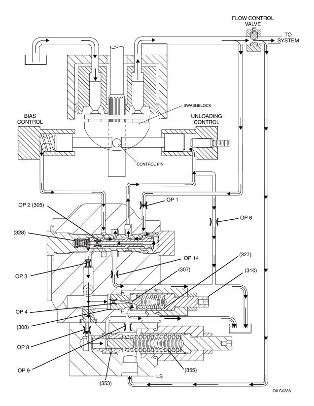
Figure 6. Compensating Pressure - Unloading
