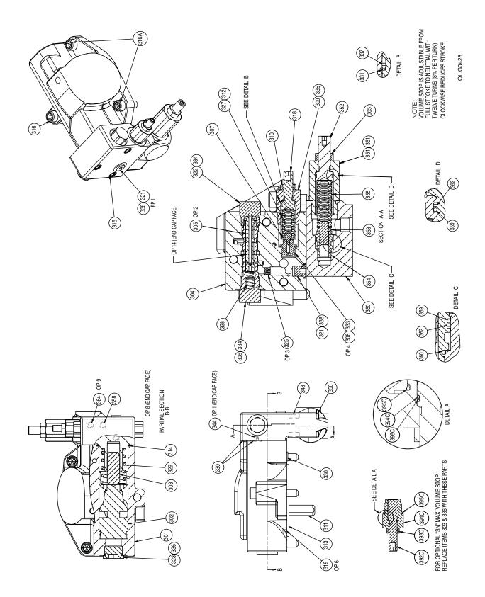
Figure 8. Cross Section Parts Drawing for "P-1NN/F" Single Pressure Compensator, Series F1U Control (517108-200 sheet 1)
