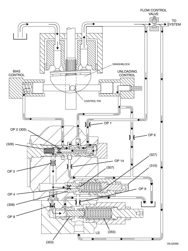
Figure 5. Load Sensing Control - Unloading
