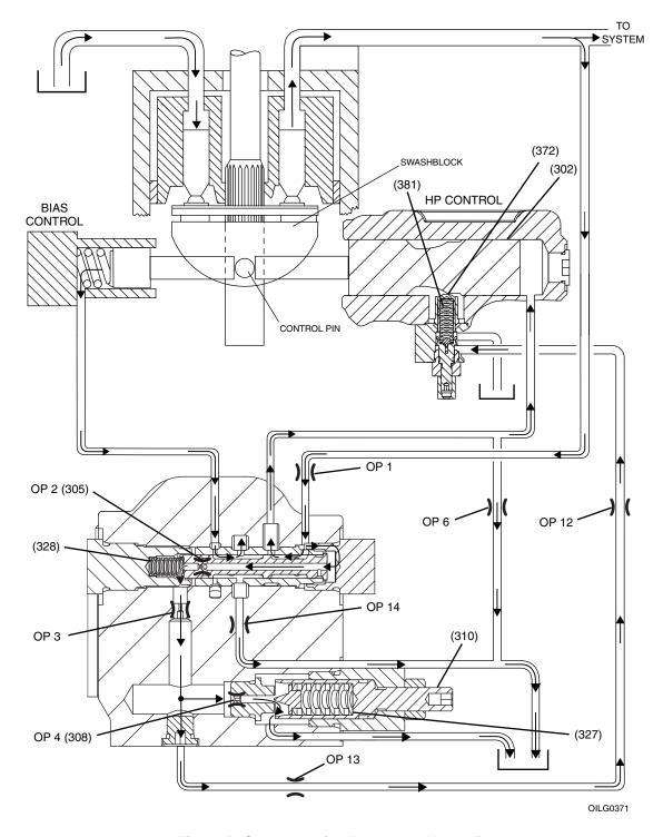
Figure 5. Compensating Pressure - Unloading
