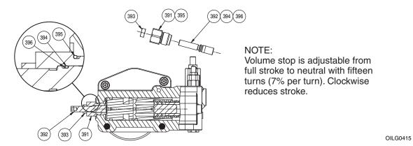
Figure 7. Exploded Parts Drawing for "P-1NN/H" Maximum Volume Stop, Series F1U Control
