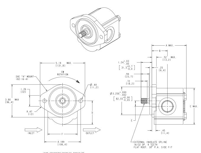
(FOR COUNTERCLOCKWISE ROTATION, INLET AND OUTLET ARE REVERSED.)
